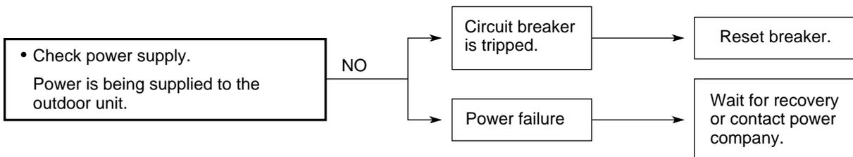
**B. Check "OPERATION selector" switch in the indoor unit.**
