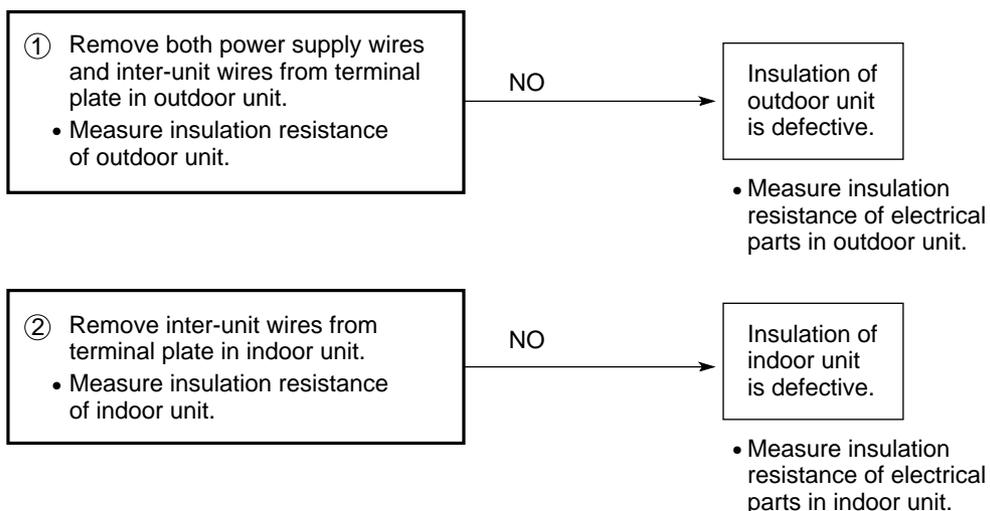
**B. Circuit breaker trips in several minutes after turning the air conditioner on.**
