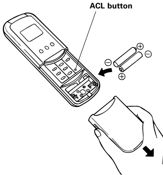
1. Slide the cover in the direction indicated by the arrow and remove it.
